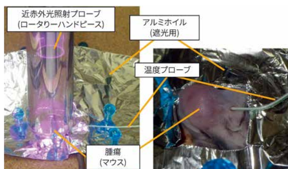
General appearance of NIR irradiation experiment after administration of liposome containing an immune activating substance.
